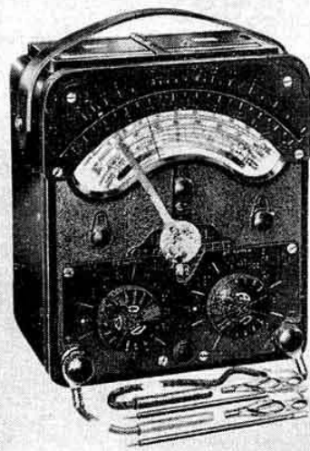
The specially adapted Avometer which has been designed for the use of blind amateurs and service men.
