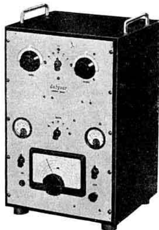
The new Labgear desk top 150 watt band-switched transmitter which occupies a base area of only 1 sq. ft. It weighs less than 50 lb. The calibrated v.f.o. dial is at the bottom of the front panel with the p.a. controls above. The cabinet is raised slightly to allow air to be drawn in for convection cooling purposes. The top is perforated to allow the warm air to escape (Photo by courtesy of Labgear (Cambridge) Ltd.)
